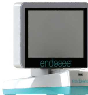
Figure 3: Display Module connected to Docking Station.
